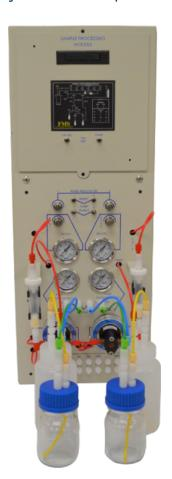
The EconoTrace System is expandable from one to four modules allowing for up to 8 samples to be run in Parallel.
