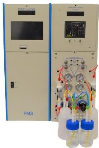
The EconoTrace 3 system runs six samples in parallel and provides direct to Centrifuge concentration.
