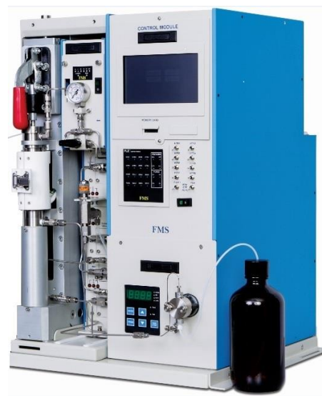
Figure 1. PLE System used for soil extraction
