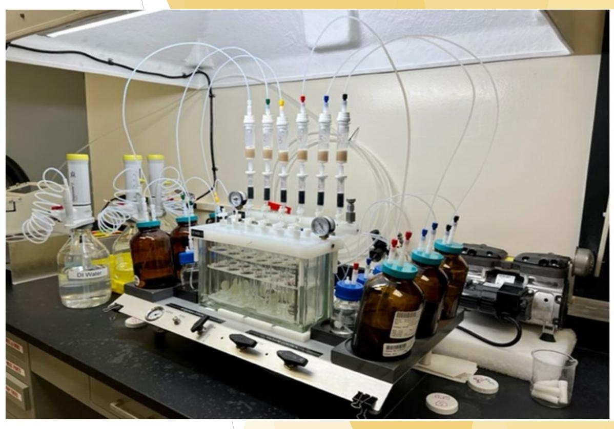
The City of San Jose (CSJ) laboratory was able to fully validate EPA methods 608.3 and 625.1 using a cartridge-based SPE. Following SPE method validation, we have analyzed industrial compliance samples, plant effluent/influent, and Performance Testing (PT) samples with great success. By extracting with SPE instead of LLE we have greatly reduced both time and solvent used by our extractions.
