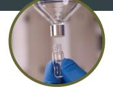
Vial Evaporator ■ Reduce sample to 10 uL final volume under 1-1.5 psi nitrogen at 25 °C
