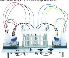
Using vacuum & nitrogen, the EZPAC automatically loads the samples, rinses the sample bottle and delivers the solvent to the SPE cartridges. The final extract is delivered directly to the extract vial ready for final concentration in the FMS SuperVap®. The process saves both labor and time.
