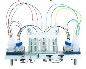
Using vacuum & nitrogen, the EZPAC automatically loads the samples, rinses the sample bottle and delivers the solvent to the SPE cartridges. The final extract is delivered directly to the extract vial ready for final concentration in the FMS SuperVap<sup>®</sup>. The process saves both labor and time.
