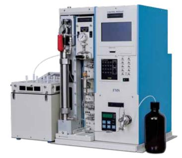
A single module PLE sending oil from 2 ounces of flower extracted directly to a SuperVap® Concentrator. Capable of processing 4 lbs. in 8 hrs.
