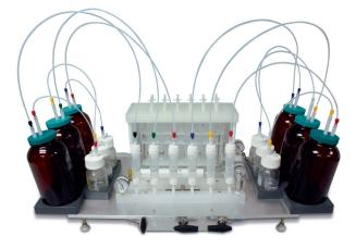
Using vacuum & nitrogen, the EZSpe automatically loads the samples, rinses the sample bottle and delivers the solvent to the SPE cartridges. The analytes of interest are extracted and then dried using a sodium sulfate cartridge to remove all water. The final extract can be delivered directly to the "Direct to GC vial Vessel" ready for final concentration in the FMS SuperVap<sup>®</sup>. The process saves both labor and time.
