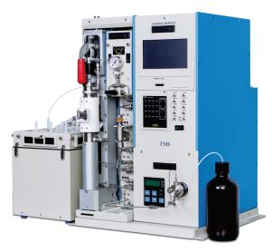
A single module PLE sending the extract directly to a SuperVap® Concentrator
