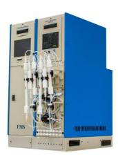
EconoPrep® Multi-column Sample Cleanup system is modular, it runs two samples per module, supports up to 4 modules to run a total of 8 samples in parallel.
